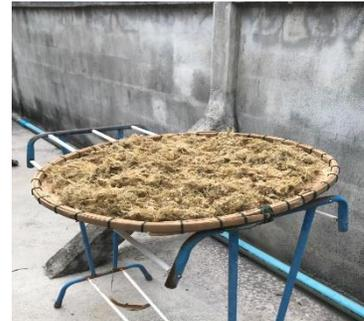
**Figure 3** Sun dry frayed fiber for 2 days
