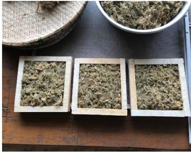
**Figure 4** Blady-grass fiber binding with natural latex in the mold
