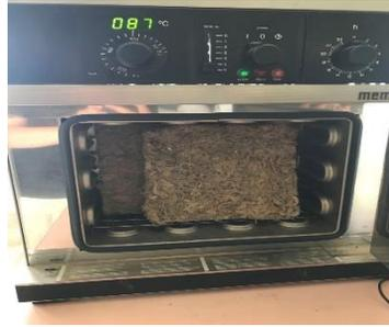
**Figure 5** Blady-grass insulation plate dry in the hot air oven at 100°C
